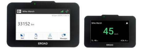
When driving, current speed, sharp braking, hard cornering and prolonged engine idling will be displayed. Colour-coding reflects increased risk associated with speed. At the end of your trip, you can see your score.
