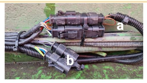
a) Shorting Pin 1 for power. b) Protect unused terminators with blanking pins AND plugs.
