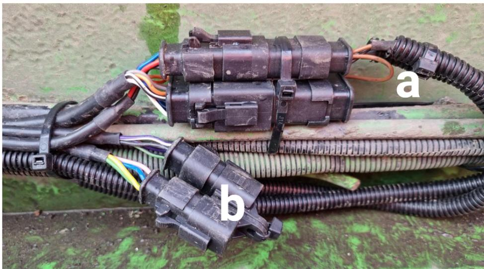
a) Shorting Pin 1 for power. b) Protect unused terminators with blanking pins AND plugs.
