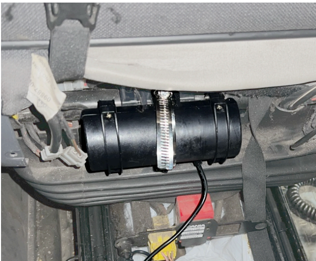
Seatshaker mounted to chair's steel strut bar, ABOVE the airseat.
