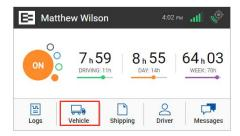
2. Tap the **Add Trailer** + Add Trailer link on the Vehicle screen. The Trailers screen displays a list of trailers previously entered.
